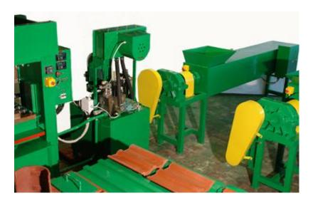
**The production line to manufacture resin-bonded products** (hereinafter referred to as **line**) incorporates equipment for manufacture of resin bonded products. The equipment is designed to produce roof, tiles, ridge tiles, paving slabs and other resin bonded products.
